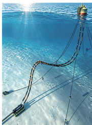
懒S型/陡S型软管 GS84212-LT/SS Lazy-S / Steep-S GS84112-LT/SS
